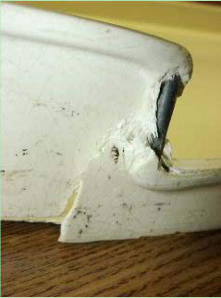
Broken tray releasing glass fiber contamination
