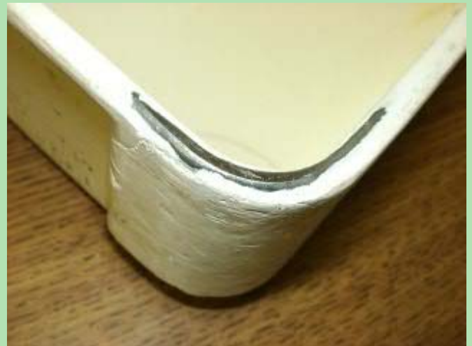
Worn out edges expose unsanitary bare metal frame
